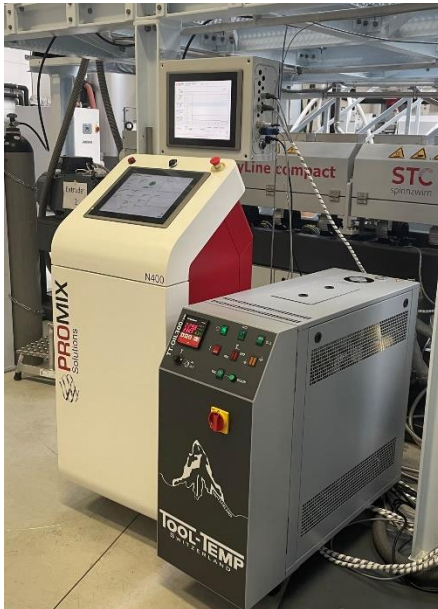
Fiber extrusion line from STC Spinnzwirn with Promix Microcell Technology for more voluminous artificial grass filaments
