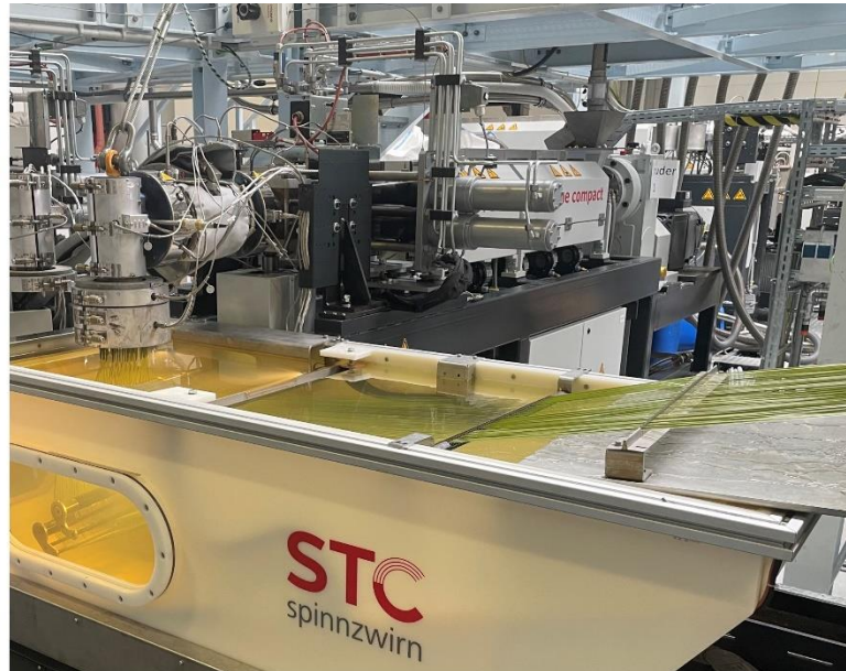
Fiber extrusion line from STC Spinnzwirn with Promix Microcell Technology for more voluminous artificial grass filaments
